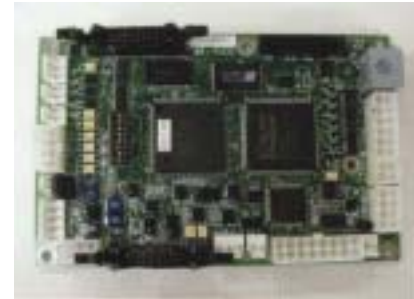
JSW original high-speed servo control board
